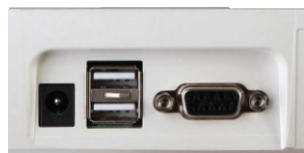
Interface for the external barcode reader, PC and lab network system Easy connect by 2 USB port
